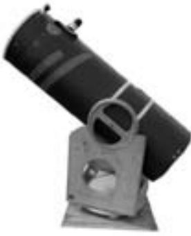
The Dobson telescope is an extremely simple and rugged large-aperture instrument and popular among amateur astronomers because of its low cost and uncomplicated production process.
